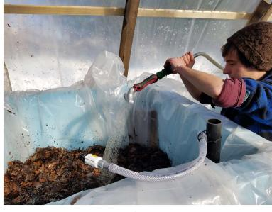
Adding pasteurized urine to leaves in experimental composting chamber.
