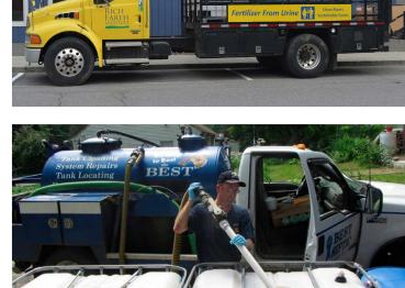
Pumping urine into a freshly-washed septage hauling tanker truck.
