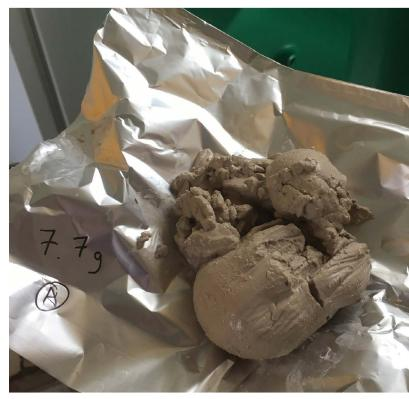
Struvite produced using urine, before drying.
