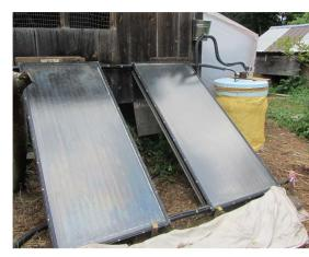
Solar pasteurizer: solar panels on left, insulated urine tank behind on right.
